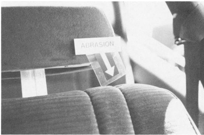
FIG. 7—In collision situations, the torso portion of the webbing can rub over the top surface of the seat back.
