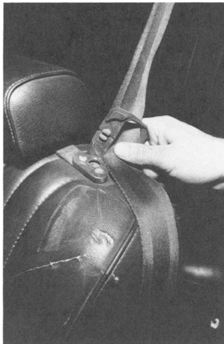
FIG. 6—During collision loading, the webbing can force the plastic guide located on the seat outboard top corner to pop out of its anchor or fracture.
