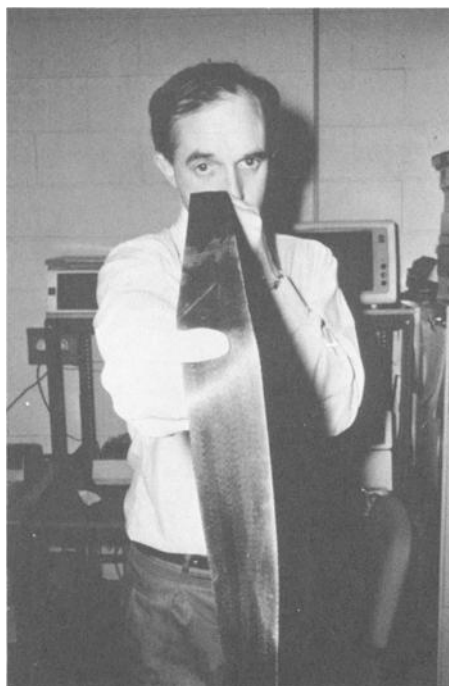
FIG. 11—Method for locating D-ring transfers on webbing.
